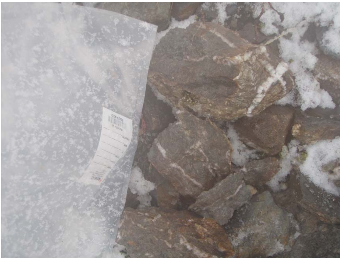
Photo 2: Rock sample 1237420 – quartzite talus at the base of an outcrop ridge with quartz stockwork and fine sulphides.
