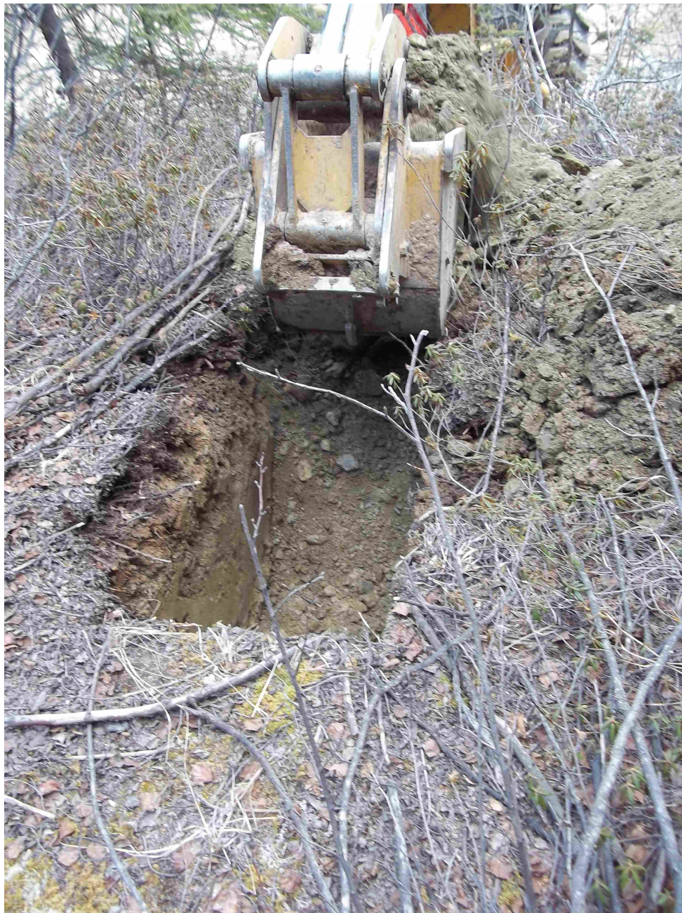
Figure 3. Backhoe Sampling. Near Green gulch - note lack of outcrop, thick vegetation, deep soil.
