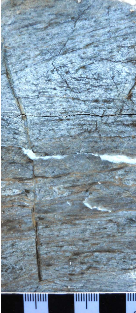
Figure 8 (DDH-10-02, 168.6m). D 2 fold in felsic schist. Not tan-coloured sericitic alteration of biotite. Note white kaolinite filling late tensile fractures.
