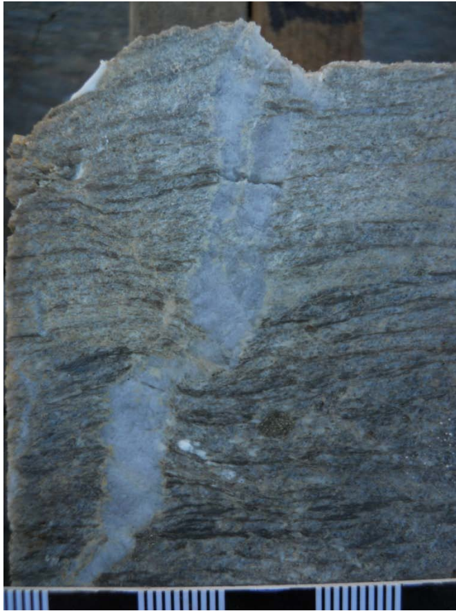
Figure3 (DDH-10-01, 130.6m) Typical D_4 kink fold in biotite schist, with a conjugate structure occupied by quartz.
