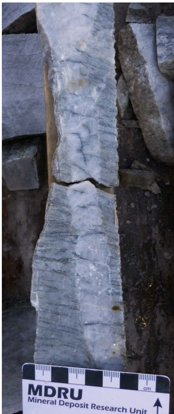
Figure 7. (DDH-10-02, 216.5m) Discordant D 4 quartz vein cut by late-generation pyritic veinlets.
