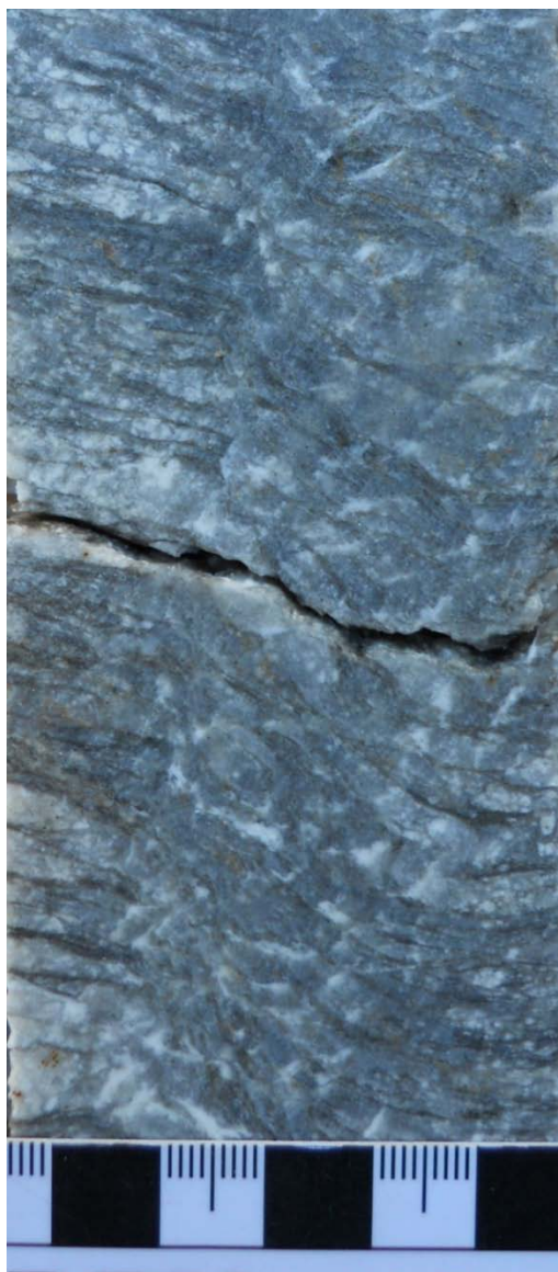
Figure 9 (DDH-10-02, 204.7m) D 4 kink zone with en echelon tensile partings filled with kaolinite (confirmed by Terraspec, D.Clark)
