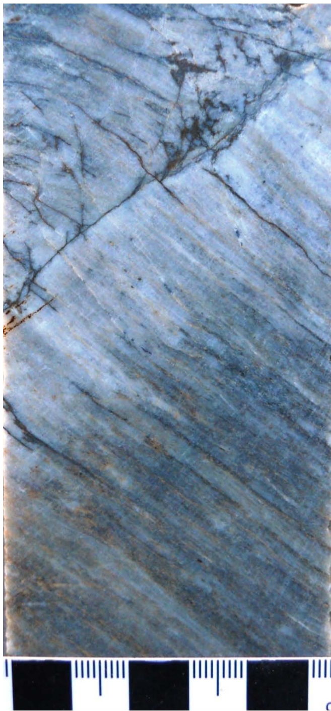
Figure 4. (DDH-10-02, 48.5m) D 4 -related zone of silicification and pyrite veinlets cutting biotite schist. Several similar features were observed in this anomalous interval (0.6 g/t Au).
