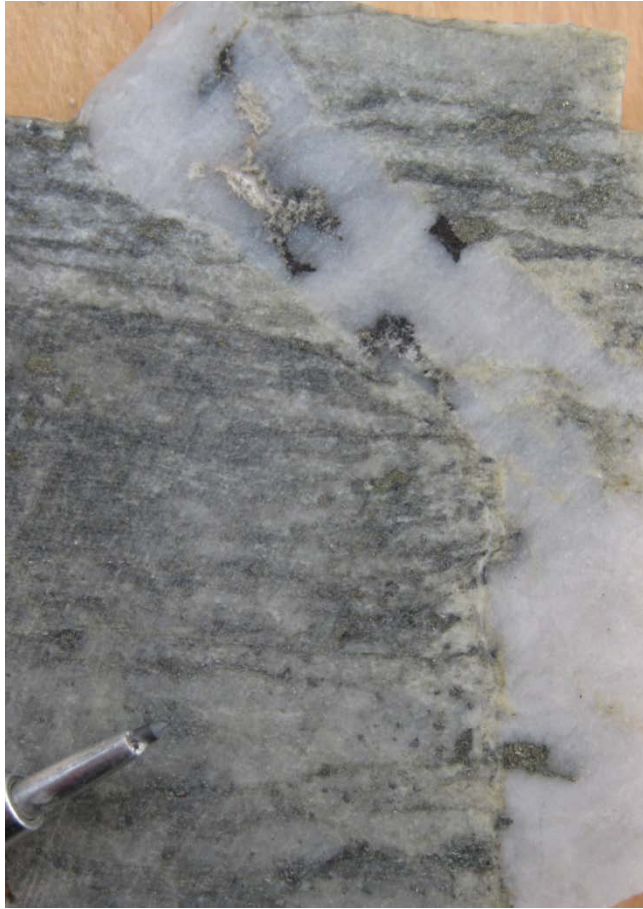
Figure 6 (DDH-10-01, 195.1m) D 4 -related quartz-pyrite-sphalerite-arsenopyrite-scheelite-carbonate vein from an interval running 2.4g/t Au.
