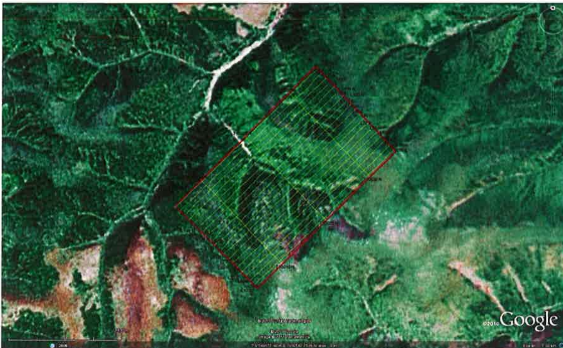
Figure 4: Block B with survey and tie lines outlined in yellow and the boundary in red in plane view.
