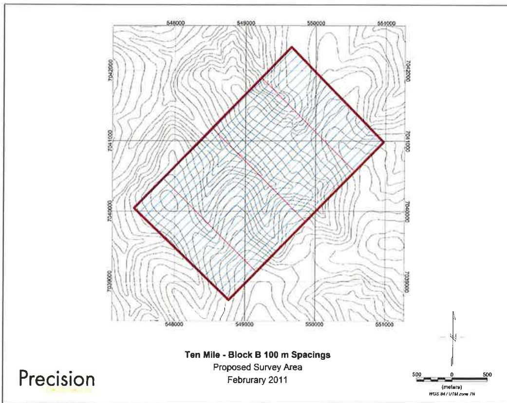
Figure 7: Proposed survey basemap of Block B showing survey and tie lines and the boundary in red.
