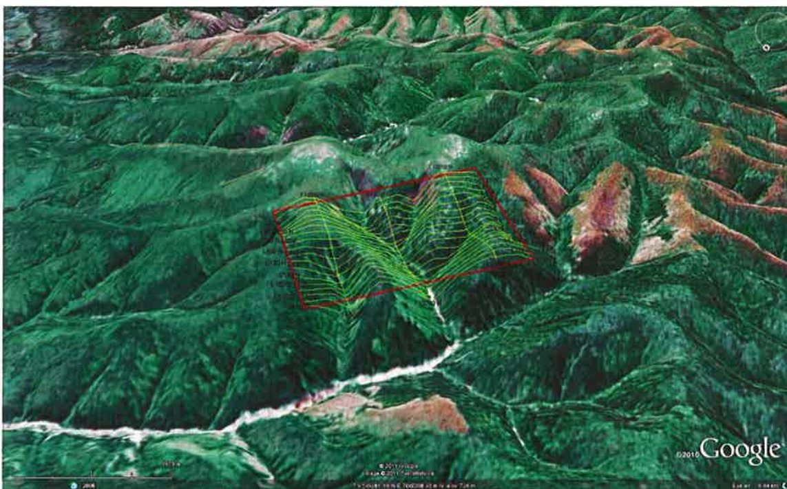
Figure 5: Block B with survey and tie lines outlined in yellow and the boundary in red in terrain view.
