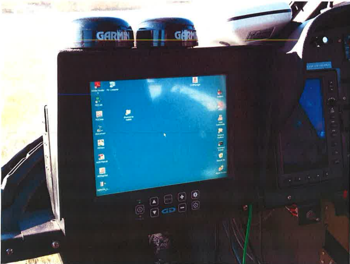
Figure 9: AGIS installed in the Eurocopter AS350 .
