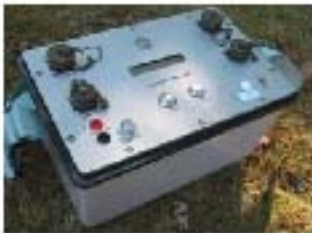
Extension Switch Pro box able to drive 21 - 48 - 72 or 96 electrodes
