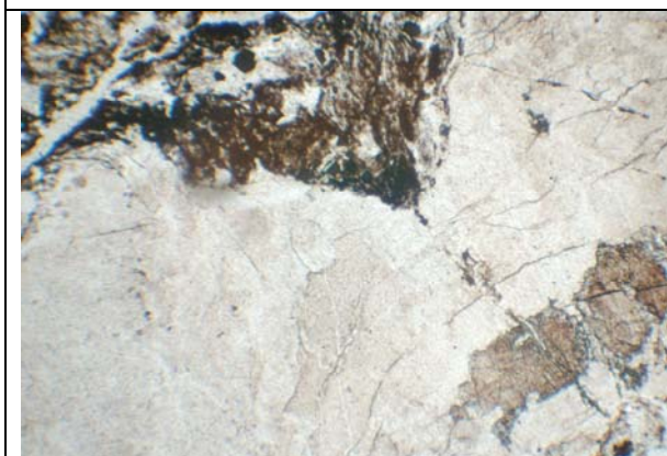
Photo 3e: There is one larger distinct deformed quartz vein in the section. It truncates foliation in the wallrock, but is also folded and strained. ppl, fov 3 mm.
