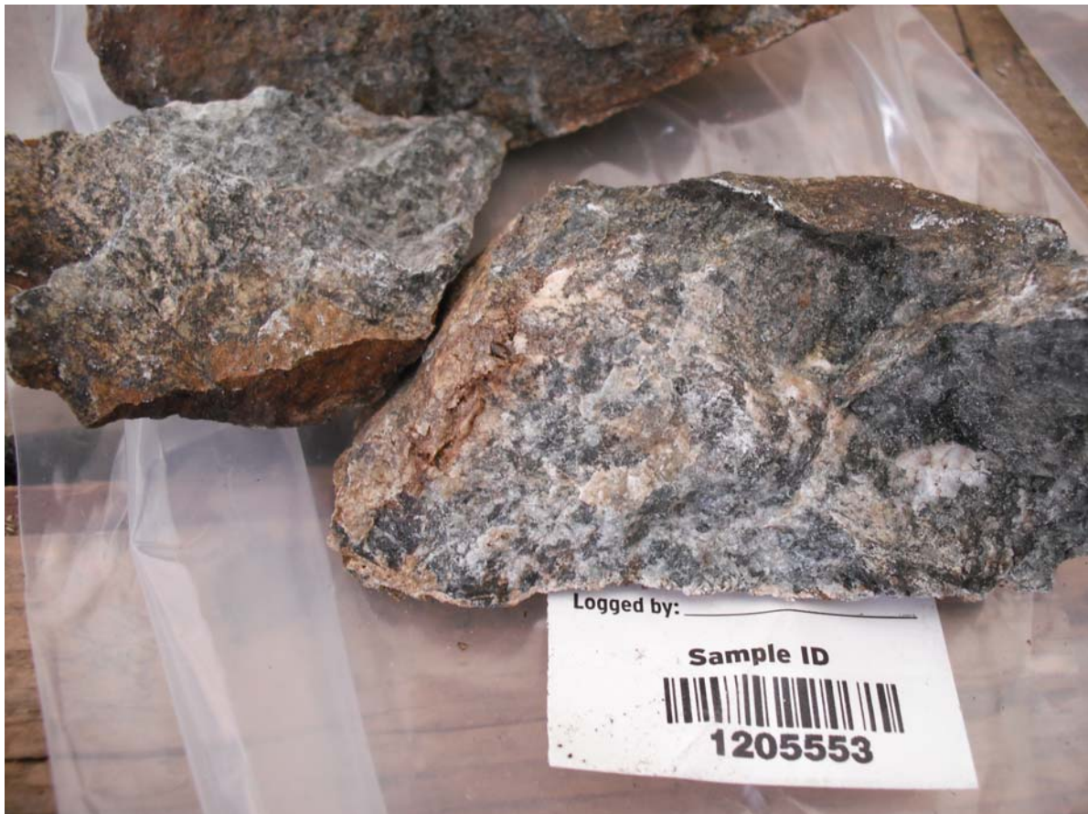
Photo 2: Sample 1205553: oxidized basalt with quartz and calcite.
