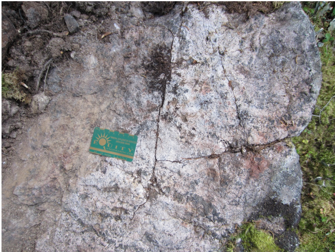
Plate 4: Sample I101906, float on the west side of COD Ridge. Rock shows patchy hematite-Mn-oxide associated with fractures in coarse-grained syenite and gave scintillometer readings up to 900 CPS.
