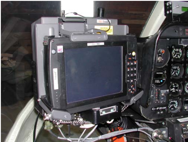
Figure 4: AGIS installed in the Bell 206.
