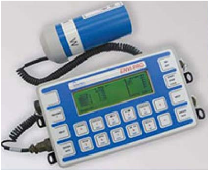
Figure 7: Scintrex Envi Pro proton precession magnetometer.
