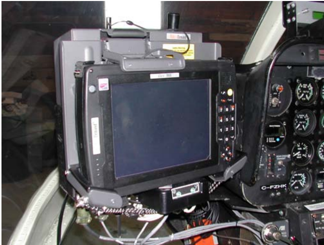
Figure 4: AGIS installed in the Bell 206.
