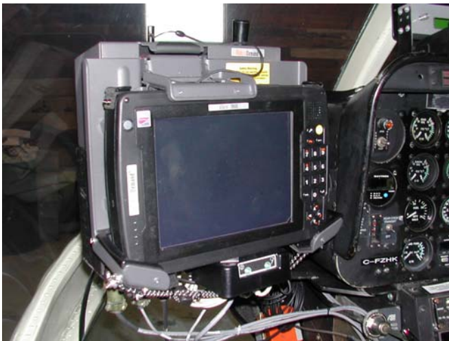
Figure 4: AGIS installed in the Bell 206.
