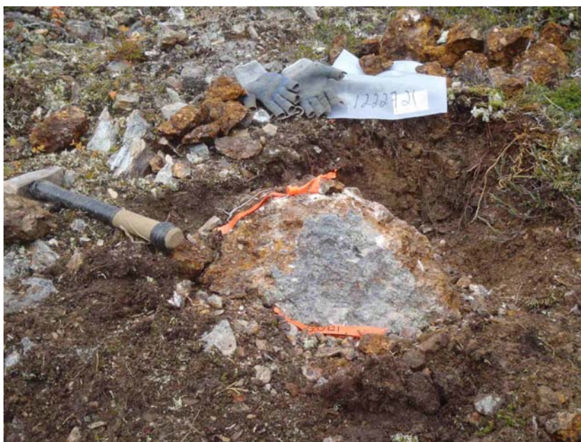
Photo 3: Area of gossan with rock sample 1222721 in subcrop. The sample carries 42 ppb Au, 31 ppm Ag, 4,392 ppm As, 89 ppm Bi, 527 ppm Cu and 5329 ppm Pb
