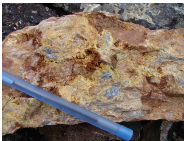
Photo 4: Moses showing, rock sample 1220635. Stibnite hosted in quartzite
