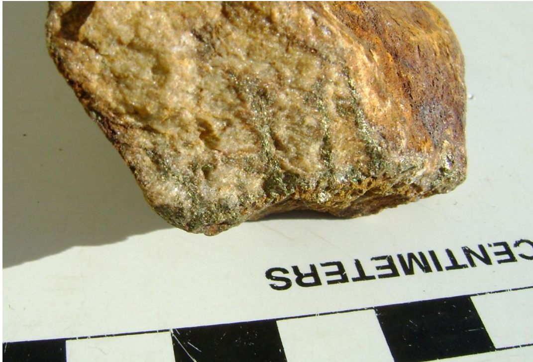
Photo 12: showing pyrite infilling fractures in silicified quartzite.
