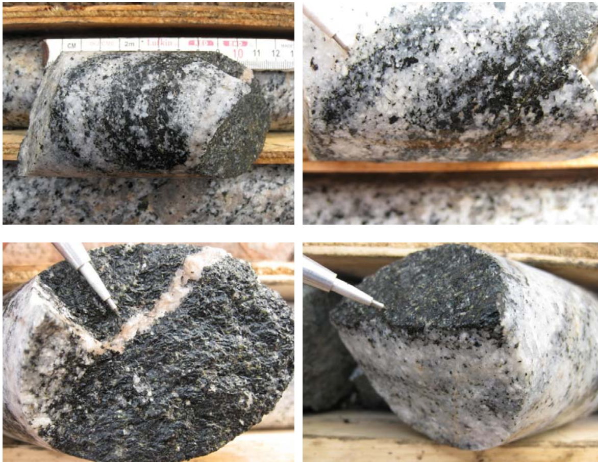
Figure 7: Strongly magnetic foliated mafic rich zones commonly associated with mineralization. These zones were intersected in KSTL-10-02 and KSTL-10-04
