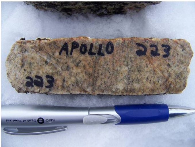
Figure 7 Granodiorite intrusion with weak mineral alignment from Site 2 at APOLLO.
