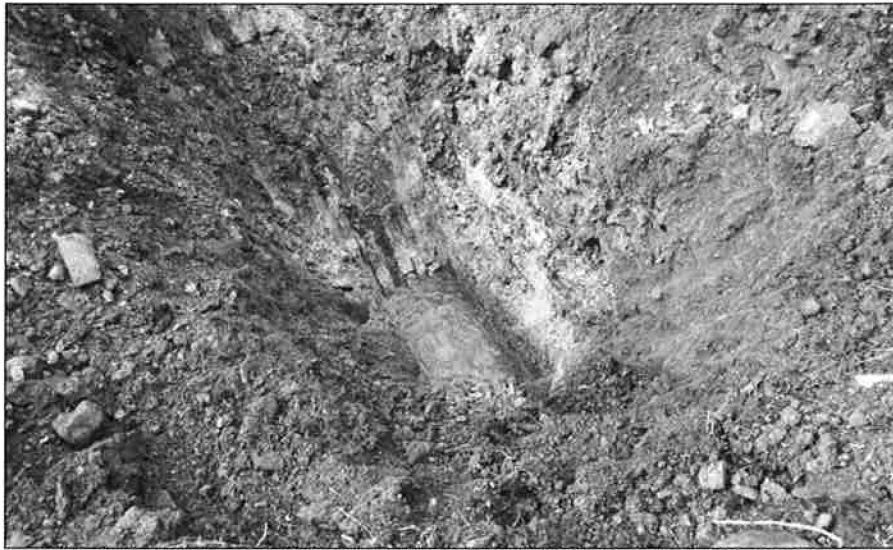
TRENCH 2: NOTE SAPROLITIC SOIL (DERIVED FROM SERICITIC SCHIST) AT BASE OF TRENCH
