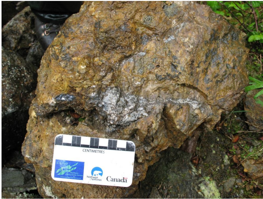
Plate 6: Mineralized boulder from the Upper Adit of the Middlecoff Zone, galena coated by anglesite(?) in a carbonate-rich breccia.
