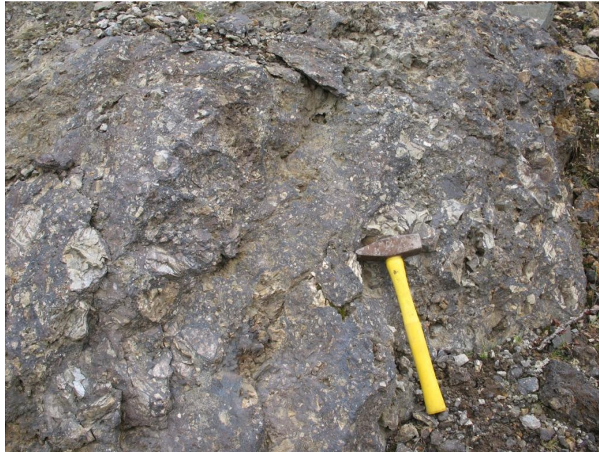
Plate 5: Breccia Zone typical of fault-related mineralization along the Main Zone in Mt. Haldane Vein system. Breccia fragments of quartzite are cemented by carbonate (siderite?) and strong Mn-oxides that are locally botryoidal. Hammer is 35 cm long.
