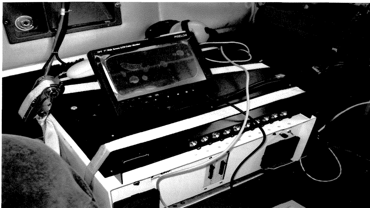
Figure 13: Fluxgeo Data Acquisition System installed in C-GPVN (2006)
