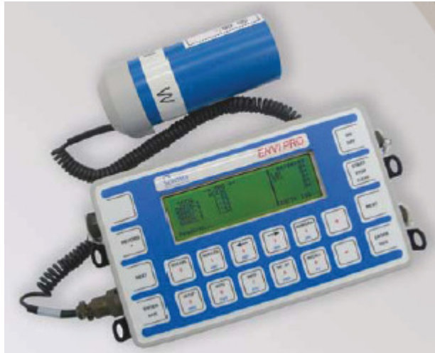
Figure 12: Scintrex Envi Pro proton precession magnetometer.
