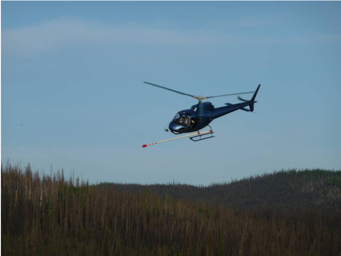
Figure 8: Eurocopter AS350 equipped with mag stinger for magnetic data acquisition.
