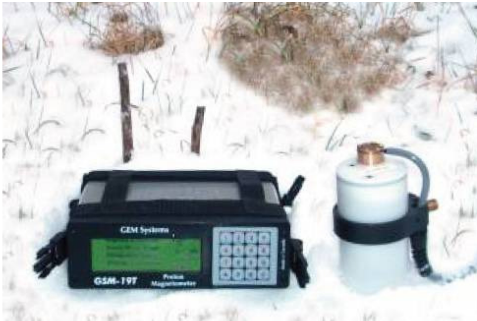
Figure 13: GEM GSM-19T proton precession magnetometer.
