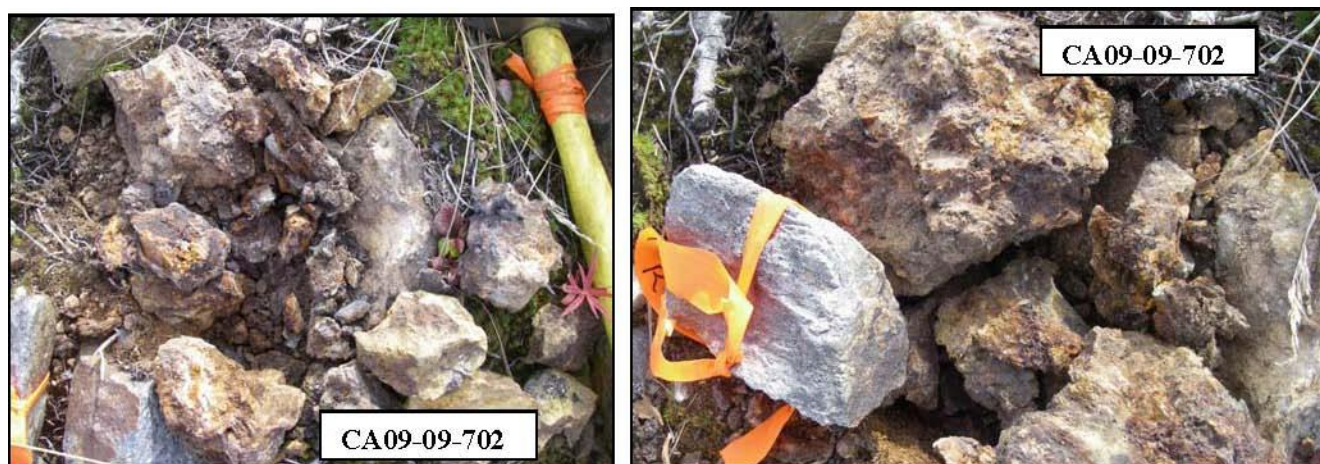
Photos 4.1. Limonite/goethite-silica breccia (Assay sample # EUCA09R-001 ; Labeled as TCAR09-03 in the assay certificate).
