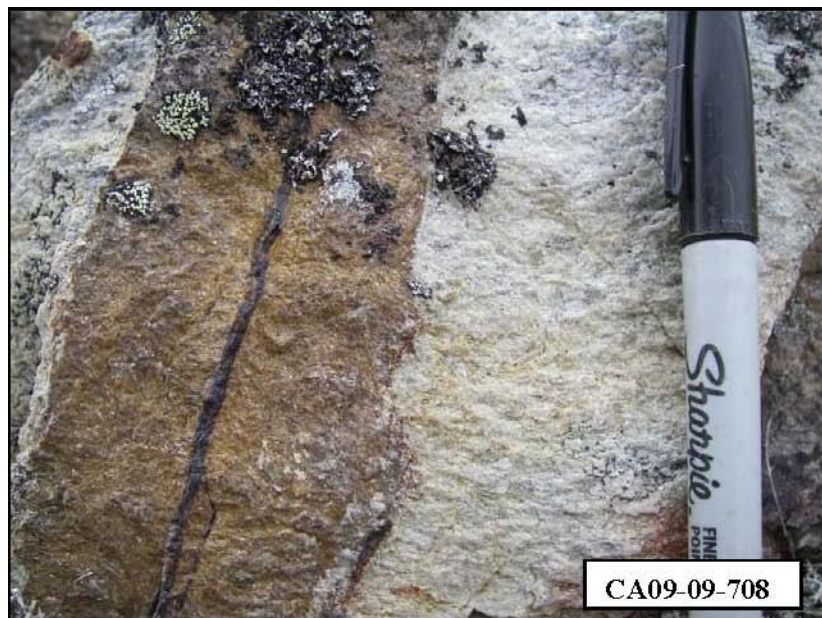
Figure 4.3. (left) Pyrite filled fracture with limonitic alteration marginal to the vein fracture (Assay sample EUGNR-09-06 ).
