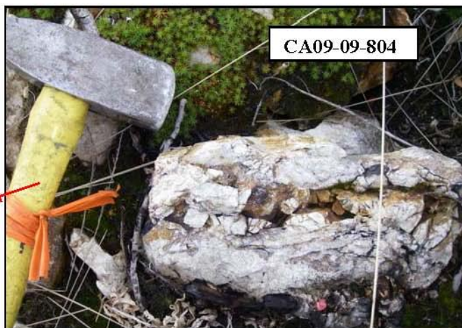
Photos 4.4. Pyrite filled fracture with limonitic alteration marginal to the vein fracture (Assay sample # MCAR-09-01 ).
