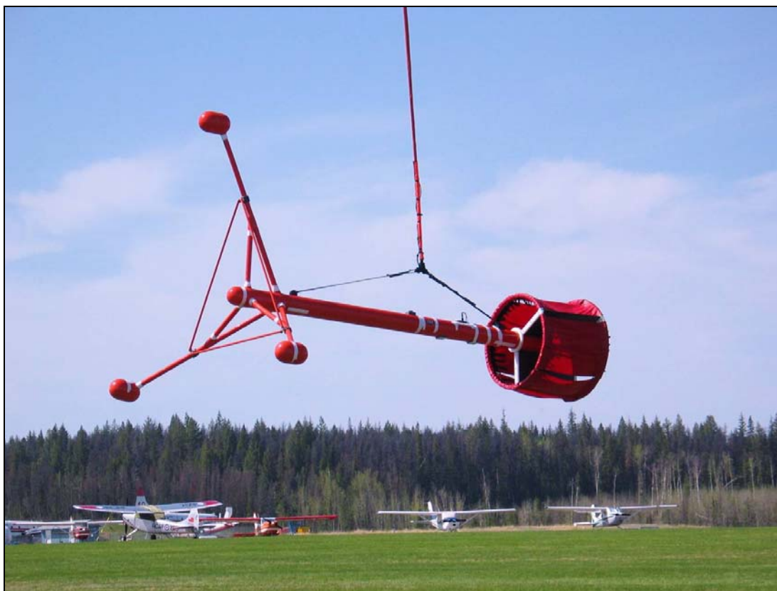
Figure 5 - The CMG tri-axial magnetic gradiometer.
