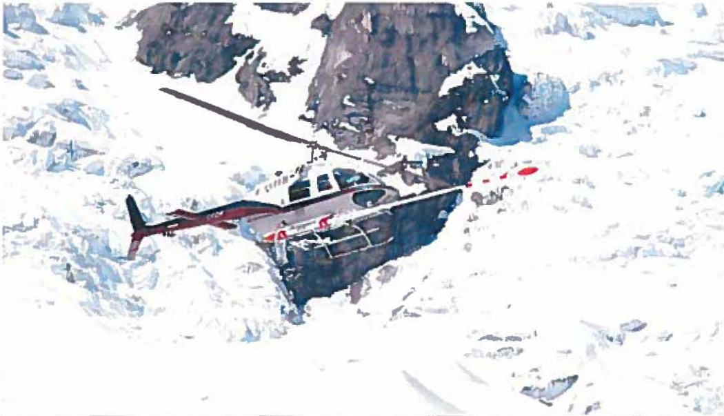
Figure 3: Bell 206 Jet Ranger equipped with mag stinger for magnetic data acquisition.
