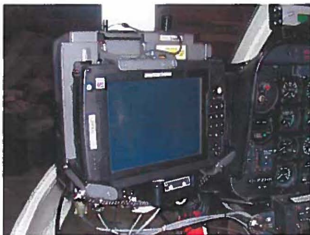
Figure 4: AGIS installed in the Bell 206.
