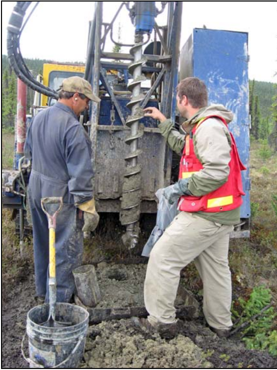
Figure 7. Collecting a bedrock rock sample from the auger flights. Sylvain Fleurant on left, Jeff Burke on right.
