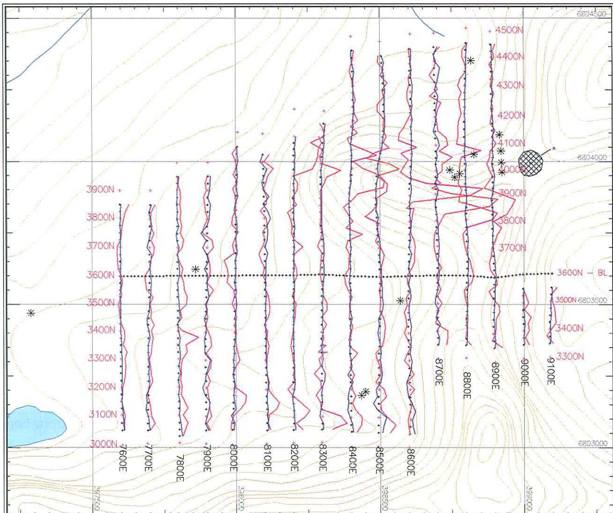
Figure 4: MaxMin 220Hz profiles. Red profiles represent the in-phase response and blue the quadrature
