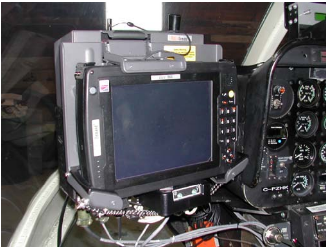
Figure 4: AGIS installed in the Bell 206.
