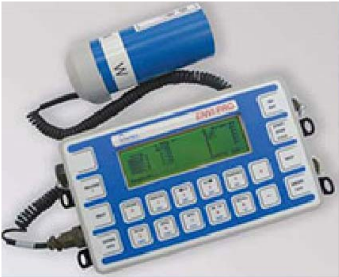
Figure 7: Scintrex Envi Pro proton precession magnetometer.
