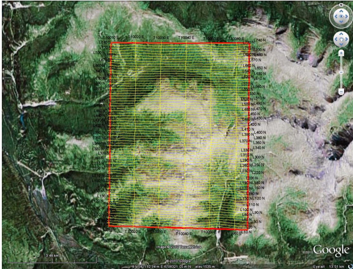
Figure 2: Survey and tie lines outlined in yellow and the boundary in red.
