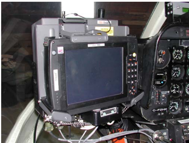
Figure 4: AGIS installed in the Bell 206.
