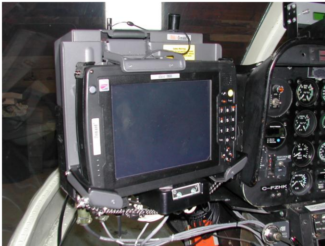
Figure 4: AGIS installed in the Bell 206.
