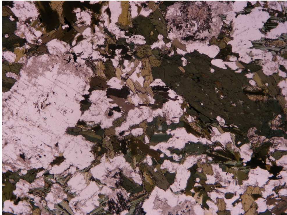
Figure 7: Photomicrographs of the (A) granodiorite and (B) diorite present in sample LON 10-5. Note the higher abundance of mafic phases (hornblende and biotite) and the porphyritic texture in the diorite. PPL, FOV = ~ 7 mm.
