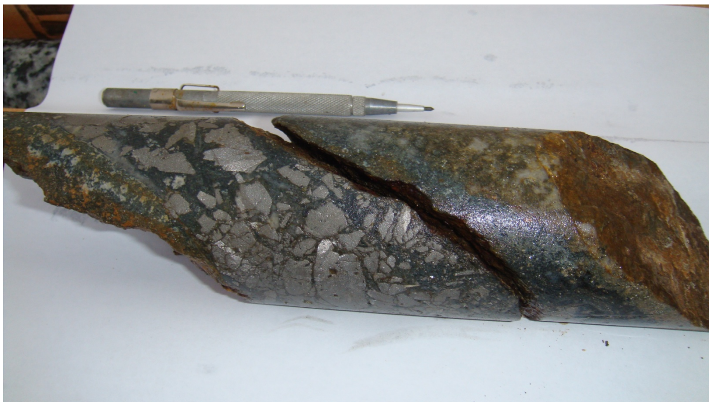
Figure 9: Brecciated arsenopyrite from LON10-04
