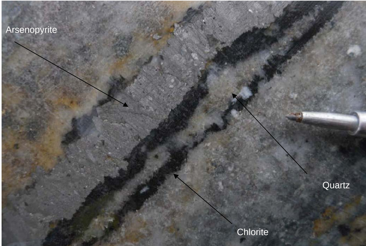
Figure 7: Arsenopyrite-quartz-chlorite vein from LON10-06
