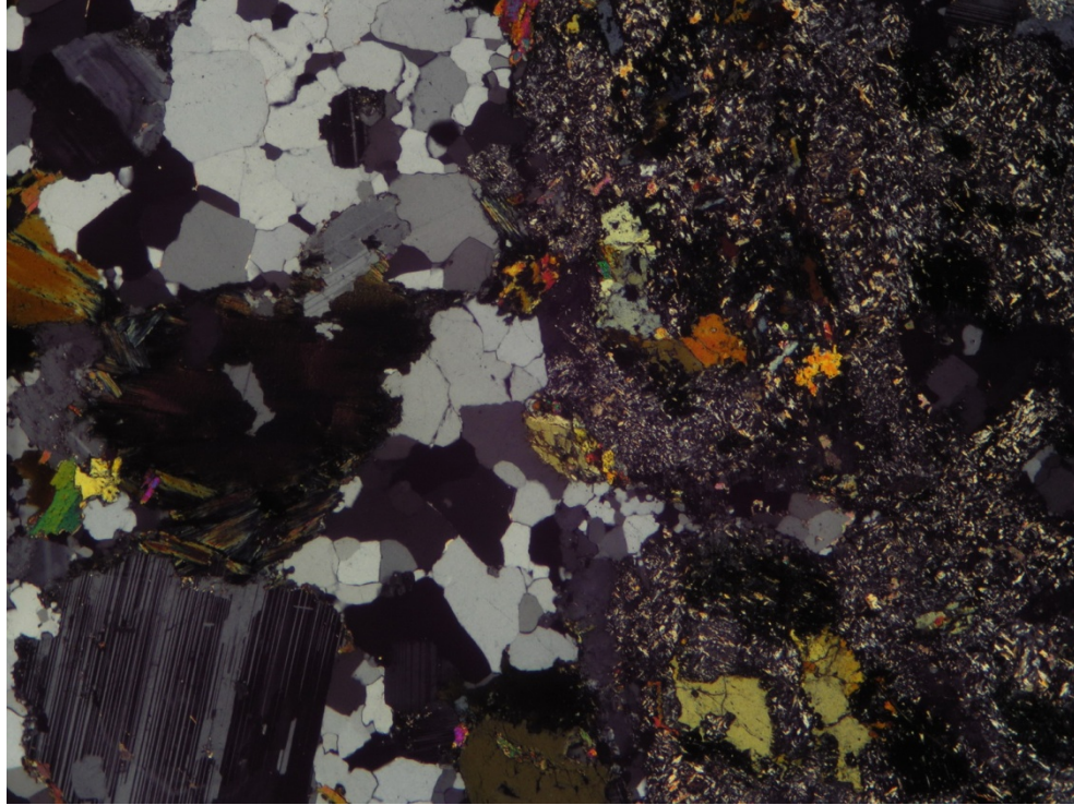
Figure 3: Photomicrograph of sample LON 10-3 showing the occurrence of unaltered plagioclase (bottom left) and partially chloritized biotite (middle left). The area shown on the right side of the photomicrograph is essentially made up of feldspar that is pitted by sericite and epidote. XPL, FOV = ~ 7 mm.
