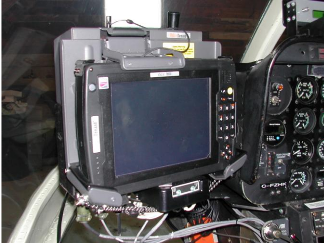
Figure 4: AGIS installed in the Bell 206.
