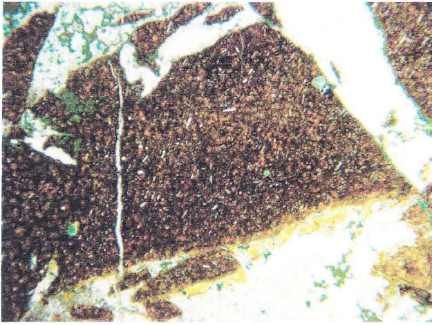
DDH08-06@203_001 FOV (mm): 6 Plane polarized light Red-brown angular fine-grained volcaniclastic clast cemented by deep green brochantite and clear carbonate- feldspar.
