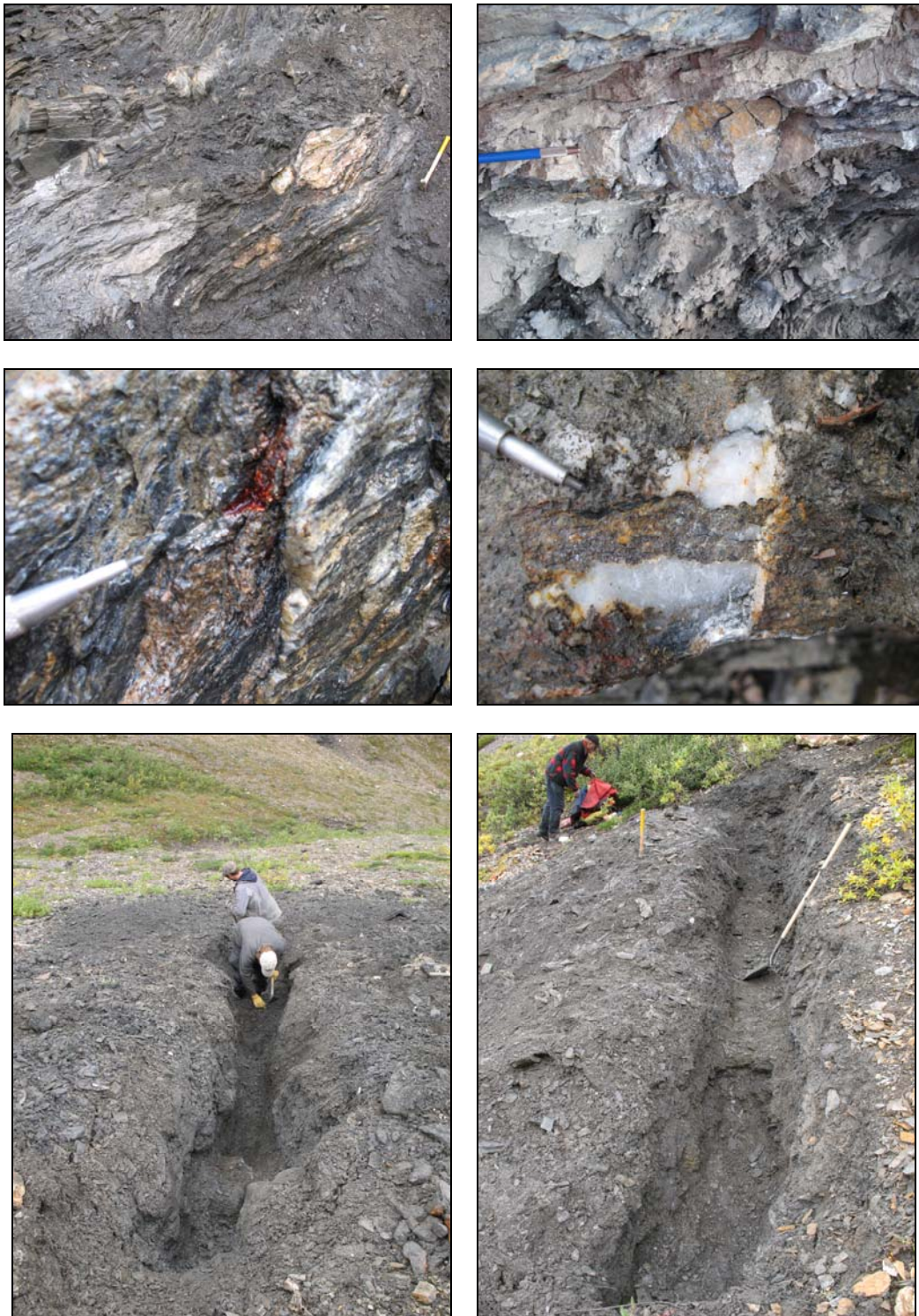
Figure 7: Keats Showing. Top left; Outcrop exposed in trench 1, buff weathering, carbonate-quartz and sphalerite foliaform veins hosted in graphitic mudstone. Top right: quartz-calcite-sphalerite pod in trench 1 outcrop. Middle left: Thin quartz-sphalerite foliaform vein in trench 1 outcrop. Middle right: Sphalerite ribbon with quartz vein. Bottom left: view from upslope of nearly completed trench 2. Bottom right: completed trench 3
