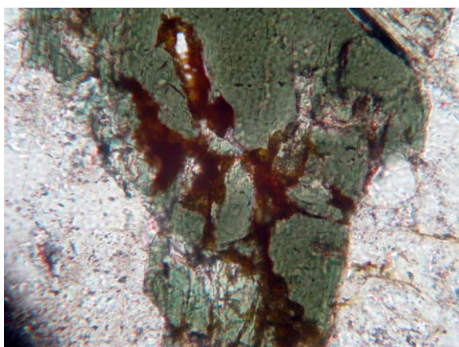
400W-A-Zone_009 FOV (mm): 0.4 Plane polarized light Orange-brown Fe-oxihydroxides partly replacing green hornblende.
