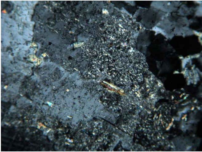
1450E-C-Zone_007 FOV (mm): 6 Crossed polars Moderate white mica (illite)+/-clay partly replacing specific growth zones plagioclase grains.
