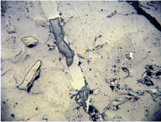
StuB-Zone-A_013 FOV (mm): 2 Reflected light. Gold(?) grain adjacent to malachite-brochantite fracture-fill veinlet.
