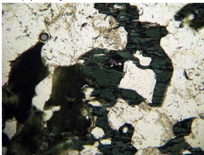
400W-A-Zone_006 FOV (mm): 1.7 Plane polarized light Green hornblende is preserved locally, but partly converted to metamorphic biotite.
