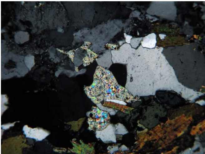
1450E-C-Zone_009 FOV (mm): 1.7 Crossed polars Malachite replaces (calcic?) portions of plagioclase grains adjacent to hornblende.
