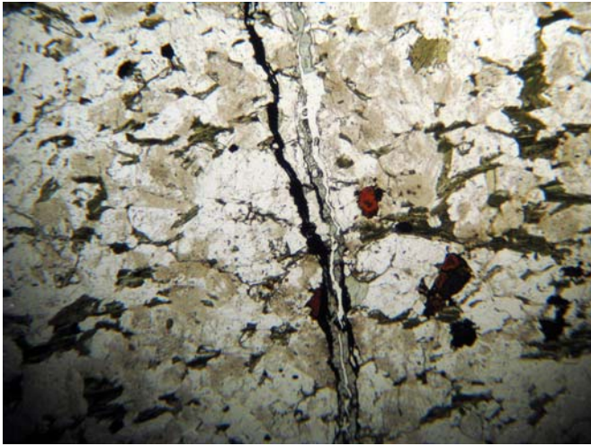
StuB-Zone-A_007 FOV (mm): 6 Plane polarized light Orange-brown Fe-oxyhydroxide along the margins of a malachite-opaque veinlet.
