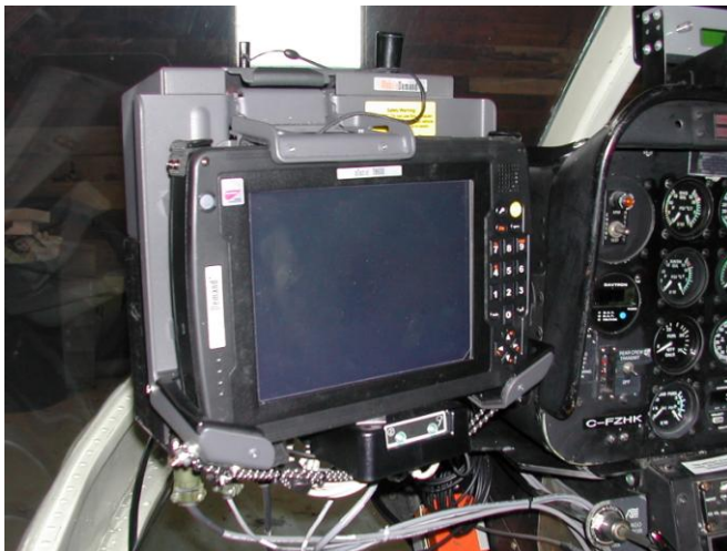
Figure 4: AGIS installed in the Bell 206.
