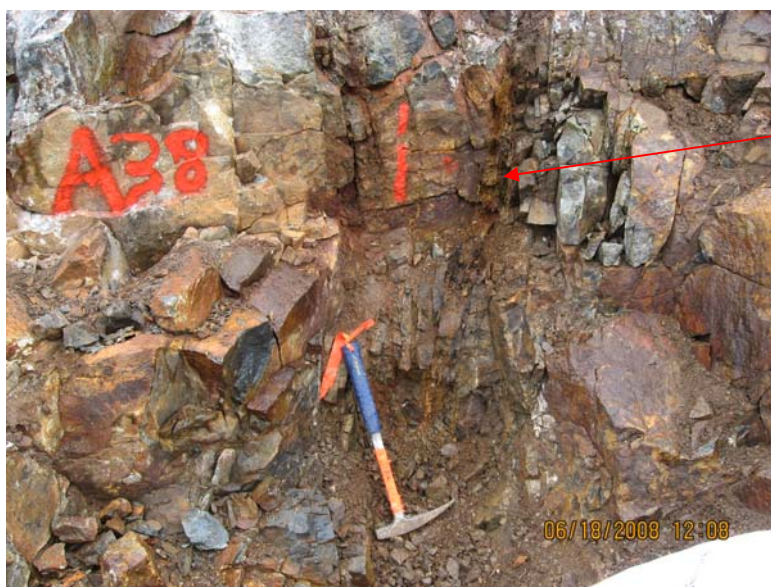
Weathered sulfide vein striking 100/80 S
