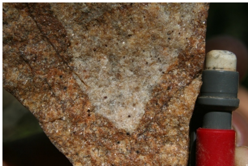
Figure 19 Disseminated, cubic pyrite in granitic dyke, Trench C, Main saddle, White property. This style of mineralisation is also seen in adjacent psammitic units. This may be related to Au bearing quartz veins found in Trench D nearby. Photo G. Corbett.
