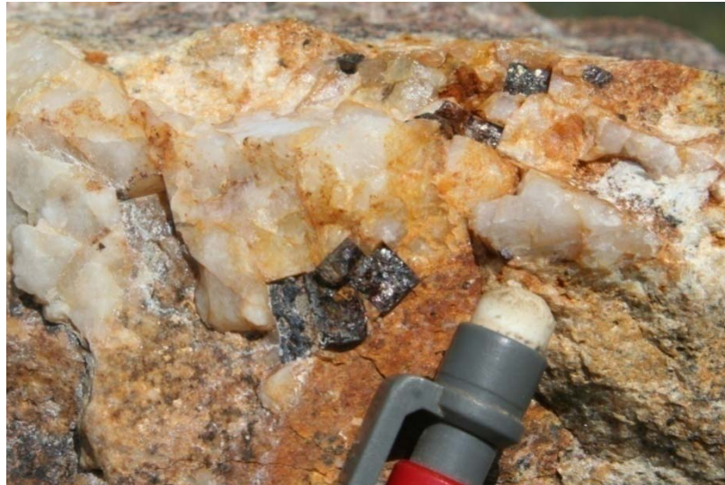
Figure 21 Galena and cubic pyrite sulphides in veining on Black Fox. Photo G.Corbett.
