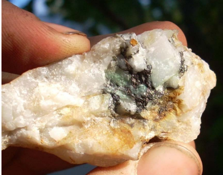
Figure 17 Sulphides in hand specimen from Trench E, the White property. This is an extension of Ryans showing along strike. Minerals include galena, chalcopyrite, malachite, and FeO staining.
