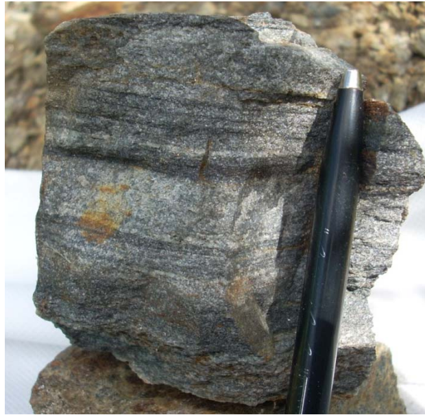
Figure 20 Grab sample from Trench A that ran 1.2 g/t Au (W063). Scorodite was observed in this sample, suggesting that at least some of the sulphide content of this rock consists of microfine arsenopyrite. It is hosted in a psammite unit.
