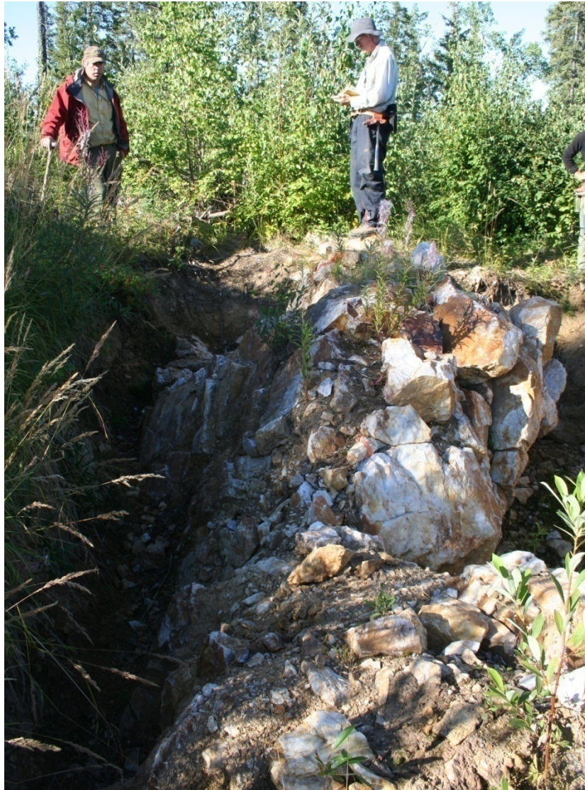
Figure 16 Ryans Showing, Shawn vein, White property. Chip samples from this vein run up to 2.1 g/t Au (Doherty & Ash, 2005). More recent grab samples run up to 10 g/t Au (WT038, Table 7). This is one of 4 veins of similar size and orientation at this locality. Furthermore a quartz vein has been exposed in a hand dug pit (Trench E) 150m to the north-east along strike that is also mineralised.
