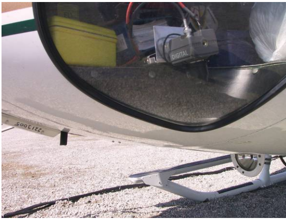
Figure 6. Digital video camera typical mounting location.
