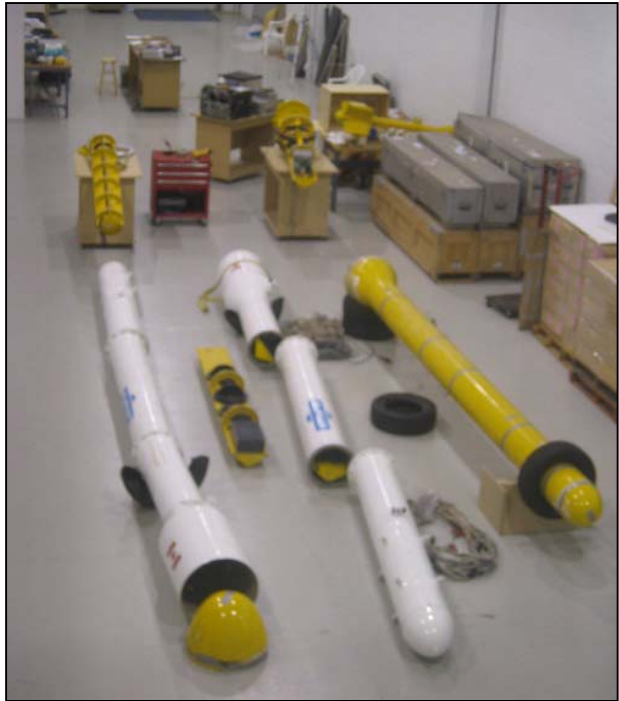
Two 5-frequency and a 4-frequency (in yellow) HUMMINGBIRD sensors undergoing preparations for the field at McPhar's offices in Newmarket, Ontario
