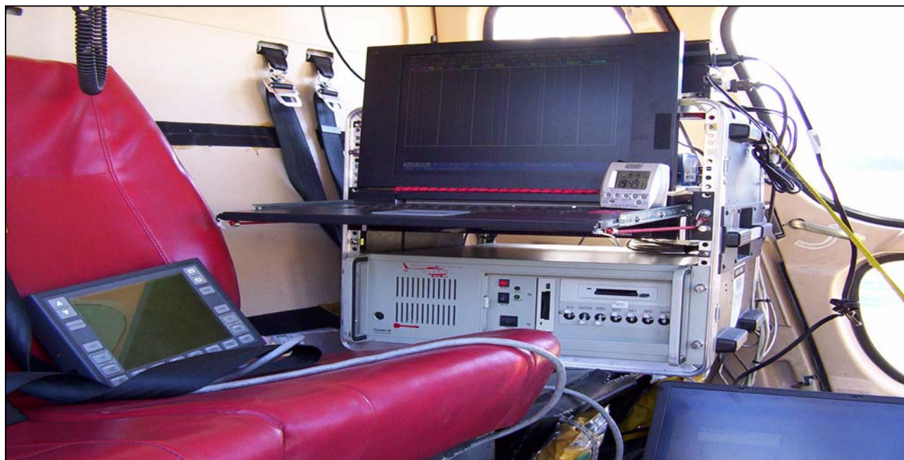
Figure 15: Geotech Hummingbird™ GDAS digital data acquisition system
