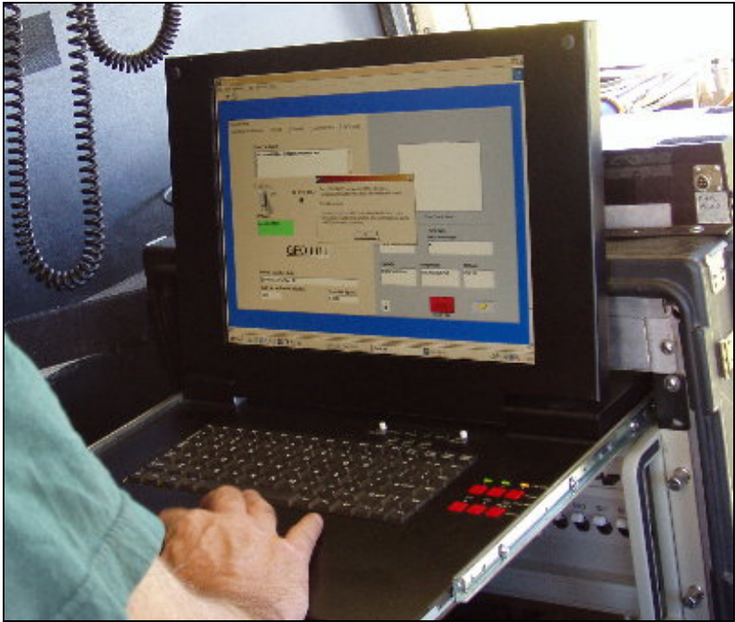
Operator's screen/keyboard assembly – HUMMINGBIRD system
