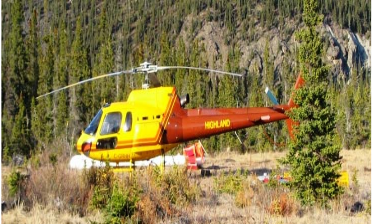
Figure 9: Survey helicopter and Hummingbird™ EM sensor at Copper Point Camp
