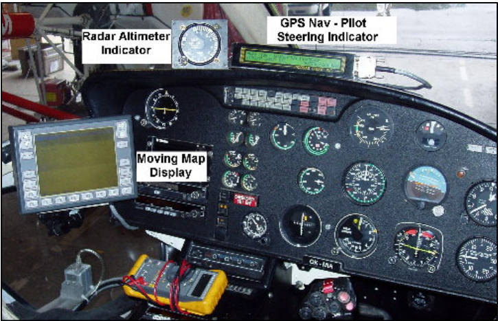
Cockpit displays for the pilot – HUMMINGBIRD system
