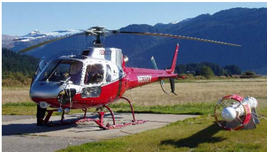
AS350B2 A-Star and HUMMINGBIRD electromagnetic sensor
