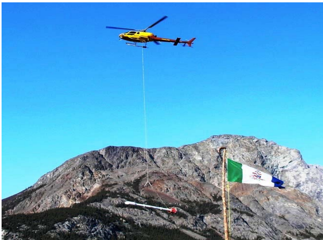
Figure 12: Survey helicopter at survey area with Hummingbird™ EM sensor
