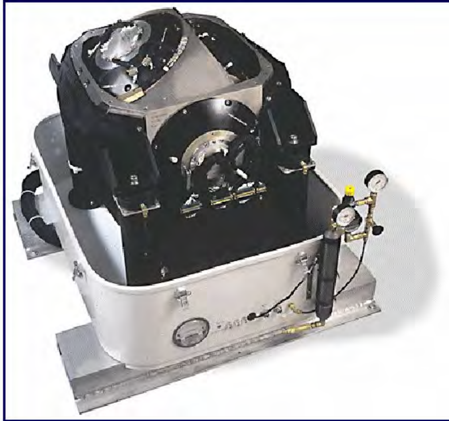
Figure 2. Bell Geospace's FTG-01 marine instrument prior to airborne conversion; support equipment not shown.
