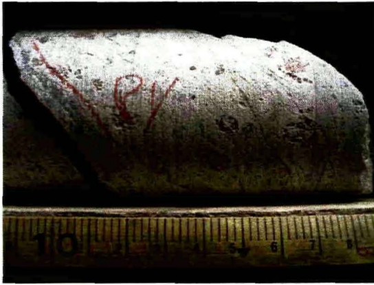
Figure 12: Intensely altered quartz-feldspar-pyroxene (amphibole) porphyry with distinctive potassium or manganese + sericite alteration
