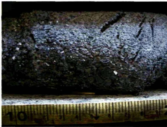
Figure 18: Fault gouge composed of lapilli tuff fragments in a felsic matrix, likely compositionally similar to the lapilli tuff
