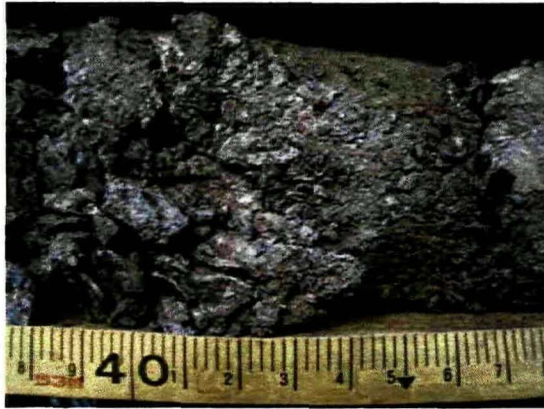
Figure 17: Carbonaceous fault gouge composed of carbonaceous argillite fragments in a carbonaceous mud
