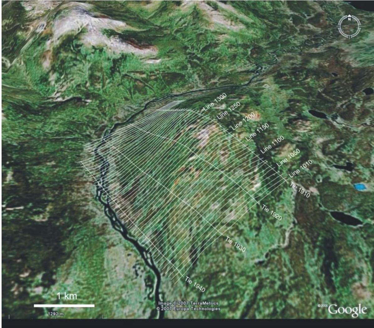
Fig. 2 Flight path showing Lines and Tie-lines superimposed on the relief satellite image.
