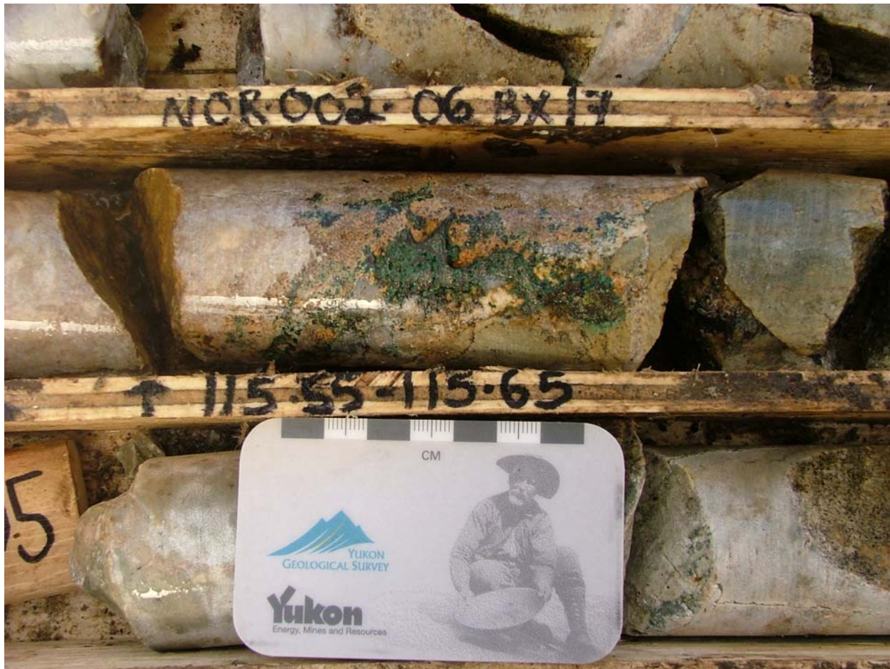
Figure 6. Clustered to dendritic chalcopyrite with malachite staining associated with carbonates-lithics \pm quartz matrix and highly to intensely carbonate-altered siltstone clasts. NOR-002-06, 115.55 to 115.65m, 1-meter sampling interval assayed 0.36% copper.
