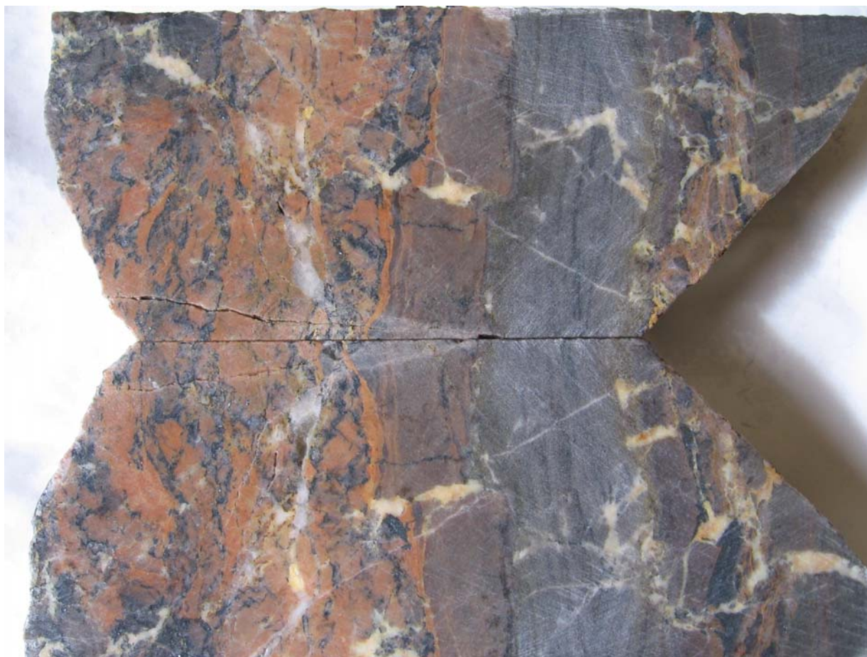
Figure 5. K-spar-hematite-magnetite-carbonate-albite altered siltstone breccia. NOR-005-06, 34 meters.
