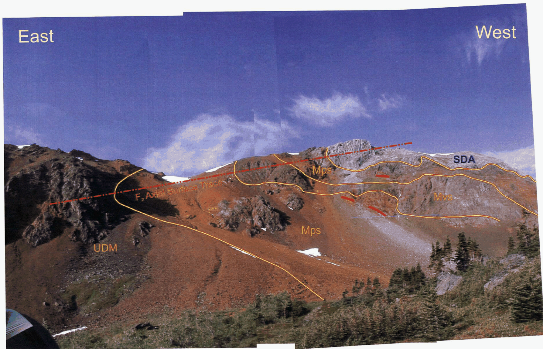
Plate 1 - Composite view, looking south, at the well exposed outcrops of the MM claims with the major map units delineated. The axial surface trace of the large-scale, recumbent F_2 fold hinge skims the ridgeline. Areas of significant mineralization (semi-massive to massive sulphides) are delineated in red. The field of view is approximately 750 meters east to west. Man, that was a nice day!
