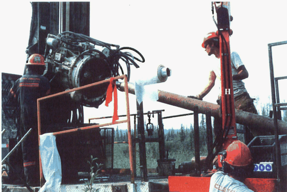
Plate 1f - Detail of the drill head tilted to receive a heavy core barrel which is slung into position with the hydraulic hoist (H).
