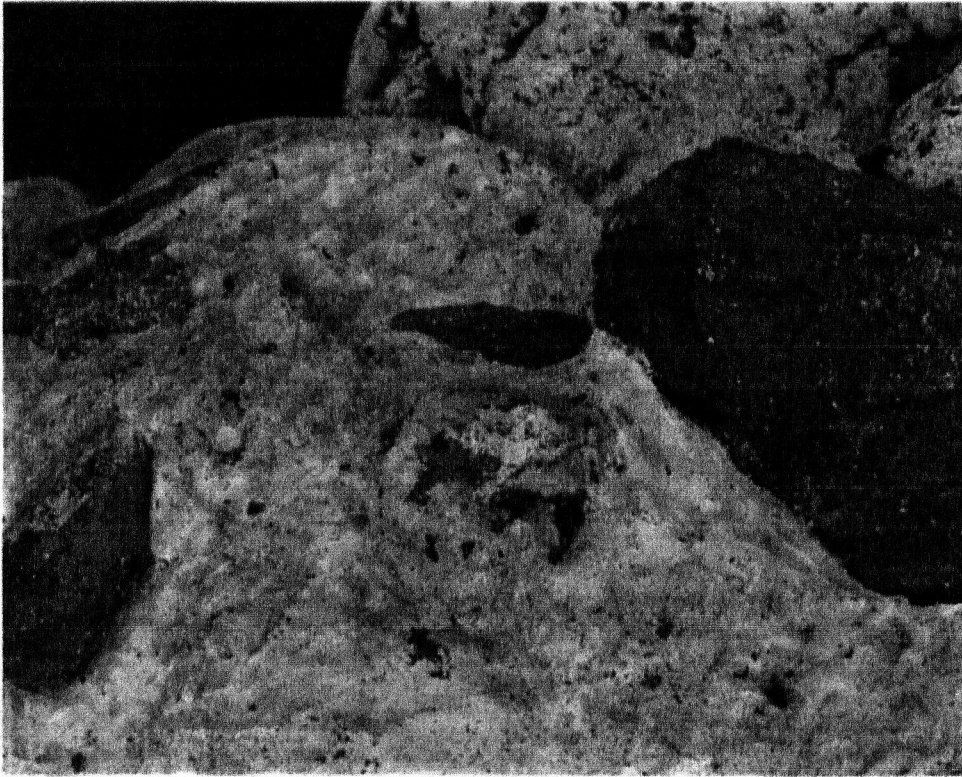
Figure 4-7. BSE image of gold-galena grains showing areas richer in Au (white) than others. FOV = ~ 1.5mm.
