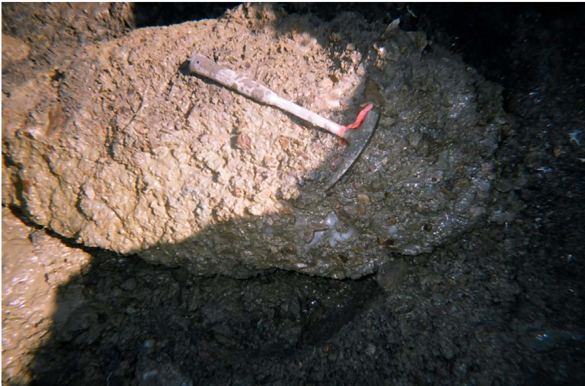
Photo 4. Flowing muck in Trench 1.
