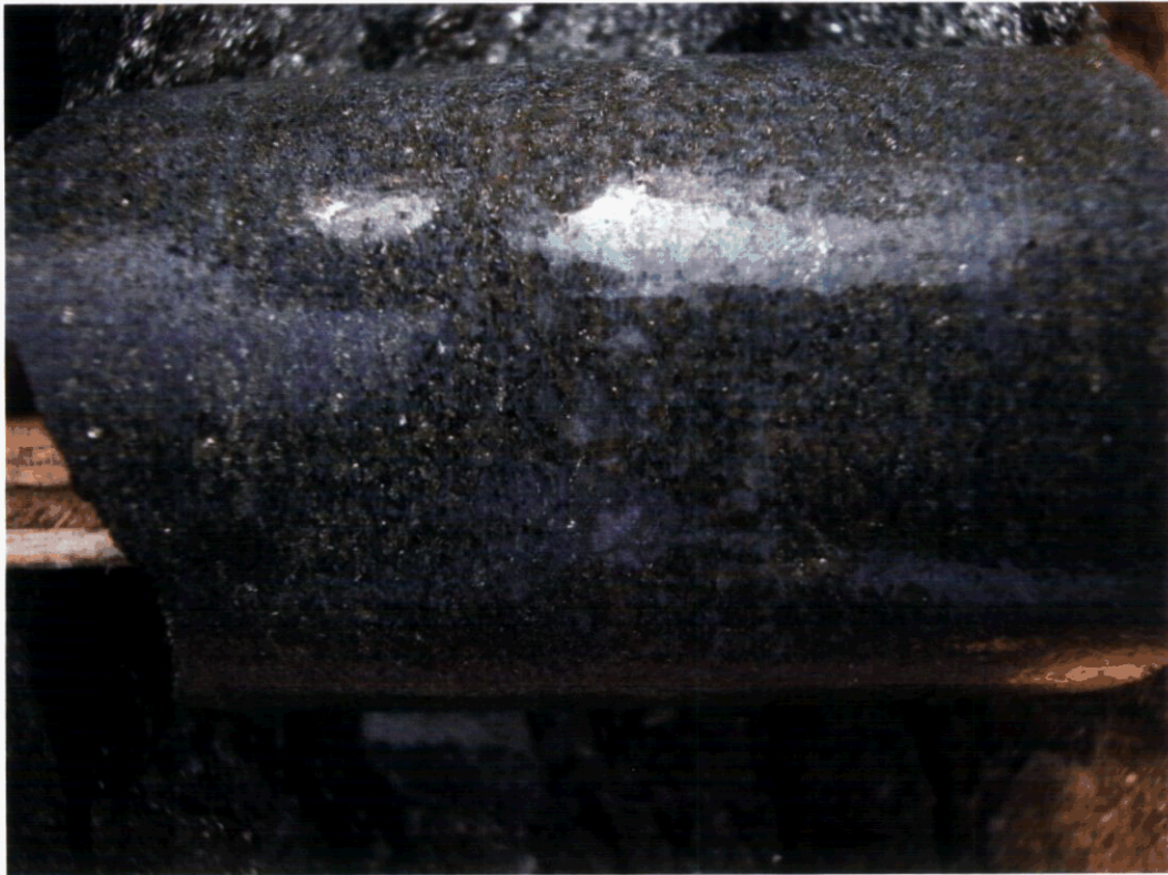
DDHM04-01 HEAVILY DISSEMINATED PYRITE 19.9-20.95m
