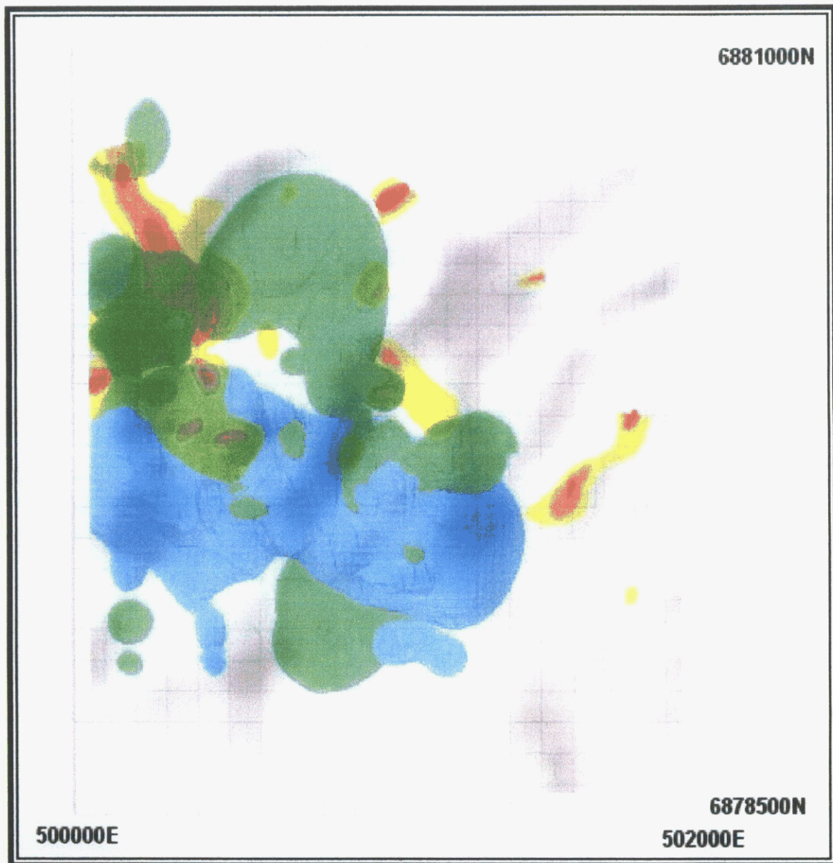
Figure 7. Plan map of gold soil geochemical survey results (red > 200 ppb, orange > 100 ppb) overlain on shaded topography. Central resistivity low (blue) and enveloping chargeability high (green) are visible beneath. Each square is 100 m x 100 m.
