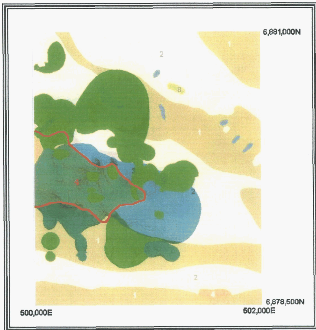
Figure 5. Top view of 3D model showing central resistivity low (blue) and enveloping chargeability high (green). Mapped contact of the altered granodiorite (Unit 4) is shown in red. The central resistivity low plunges to the east. Chargeability anomalies comprising the enveloping chargeability high are developed in both the metasediments (Unit 1) and diorite (Unit 2) surrounding the granodiorite intrusion.
