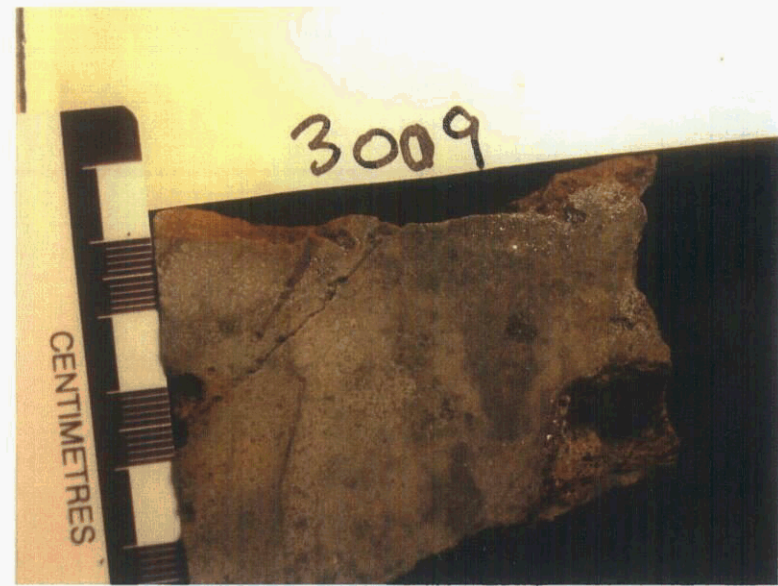
2003 sample 3009 (1457 ppb Au, 4.3 ppm Ag, 1929 ppm Cu, 188 ppm Pb, 191 ppm Zn, 148 ppm As, 6.7 ppm Bi)
