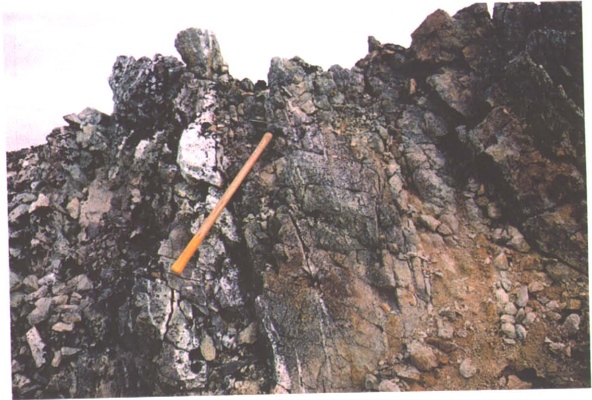
Peak Zone: sericite altered quartz-feldspar porphyry crosscut by vuggy quartz vein. Sample VR80994 across photo (30ppb Au, 8850ppm As)
