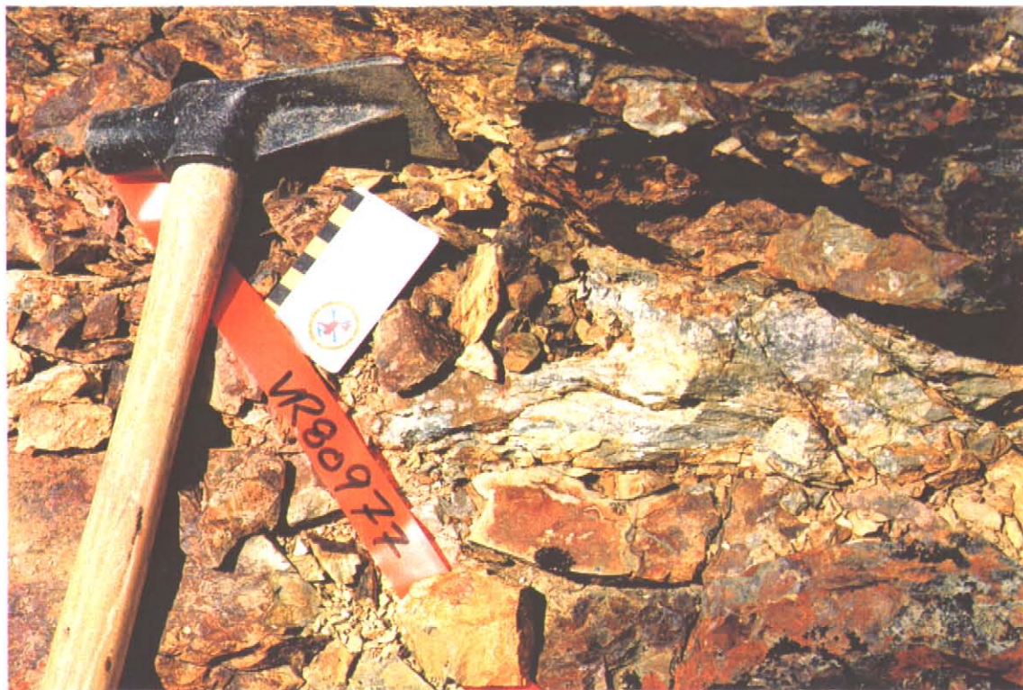
Sample VR80977 in Peak Zone. Sample returned 6.21g/t Au, >10,000ppm As, 122ppm Bi.
