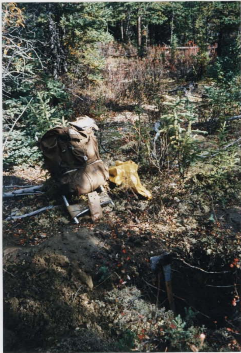
PHOTO 1 Hand dug pit at Line #2-10m West Axe handle in pit illustrates depth to base of solum and top of glacial till sample site. Looking west along cut line.
