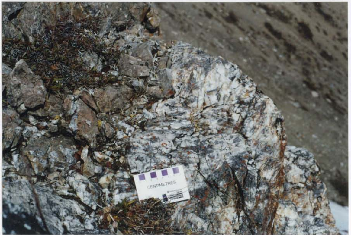
PLATE 2: Barite Vein #3; 0.80m wide with an attitude of 046/82 SE. Blue-grey colour due to carbonaceous impurities.
